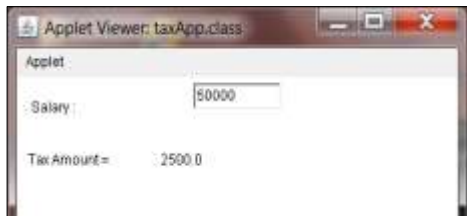
Fig. 7.9. figure shows using applet how to create a display panel like window having fixed height and width. It also shows how to input and display at particular row-column position.
