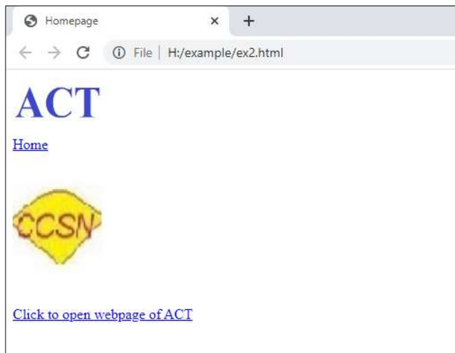
Fig. 7.2. output of a html program to show how to display any picture and how to make hyper test to link of a URL(Unified Resource Locator).
